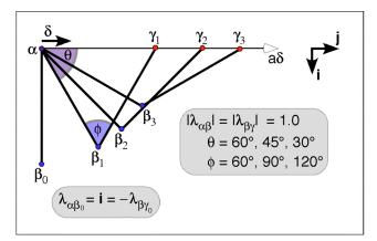
The two links are of equal length (1.0) and the initial positions for the two links are along the **i**-axis.
