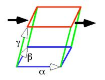
The unit cube is strained by moving the upper face relative to the lower face. This causes the  $\gamma$  edge vector to rotate with respect to the vertical to the  $\alpha\beta$ -plane.
