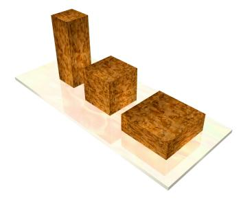
These three boxes have the same volume, therefore there is no volume strain in moving from one to the other. There is certainly strain, as is illustrated by the stretching and compression of the patterns on the sides of the front and back boxes, but it is another type of strain, linear strain.
