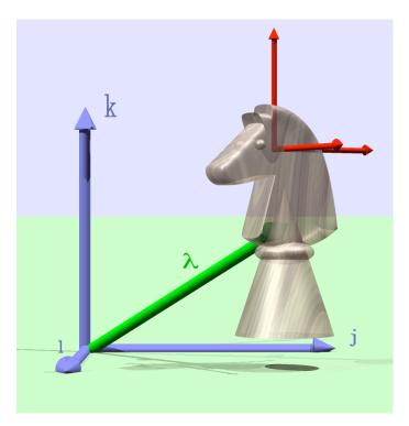
The knight is an orientable object and a frame of reference has been attached to it. The blue coordinates are the universal coordinates  $\{i, j, k\}$ . The green vector, , is the location of the knight relative to the origin of the universal coordinates and the red vectors are a frame of reference for the knight.
