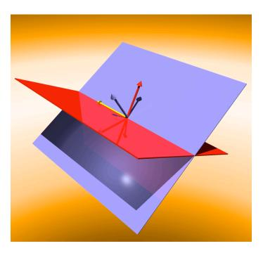
The two intersecting planes (red and blue) are formally equivalent to the vectors that are perpendicular to them (red and blue). The ratio of the vectors is the quaternion that is the intersection of the planes. The line of intersection is the vector of the intersection quaternion (yellow).
